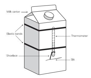
Students should secure the thermometers against the milk carton, using two elastic bands. (The thermometers should be on any two sides of the milk carton.)
