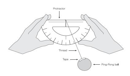
Your anemometer is now ready to use. Take it outdoors in an open area where the wind is blowing. Point the flat edge of the protractor into the wind, holding it away from your body.
